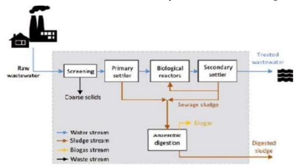
**The physical process**: this is the mechanical treatment of the water that involves removal of debris from the raw wastewater right from the point it enters the plant. The screening and primary settling of debris. Wastewater enters the treatment plant through the inlet chamber from where it is channeled to the coarse screen that removes solid waste.
